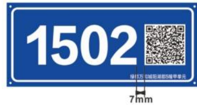
整体尺寸169x74mm 内框尺寸157x62mm 数字编号字号113pt 字间距0% 总长度97mm
