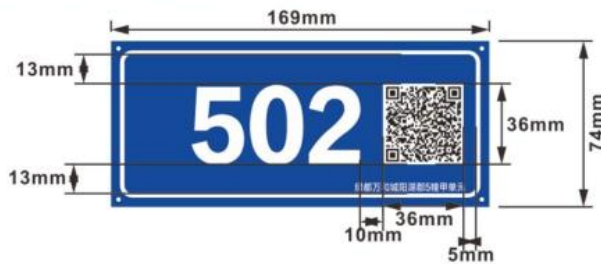
整体尺寸169x74mm 内框尺寸157x62mm 数字编号字号113pt 字间距0% 总长度76mm
